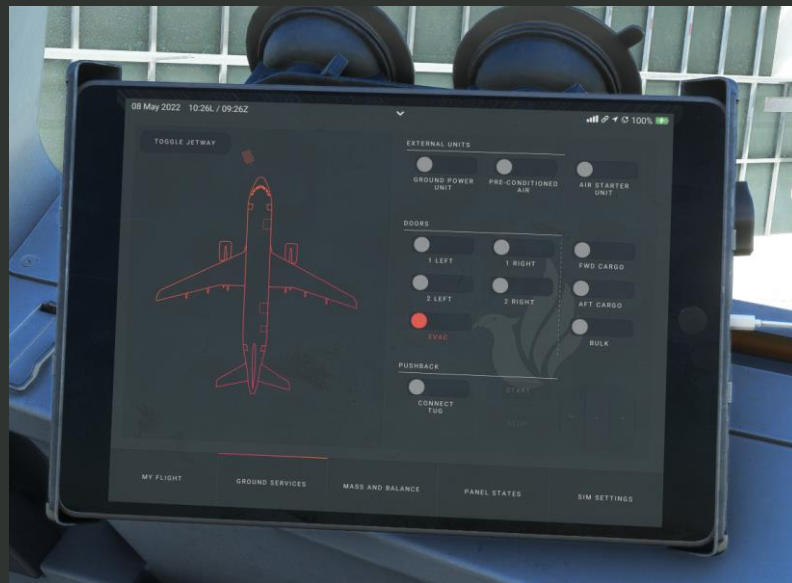
Figure 11: Ground services in the EFB
