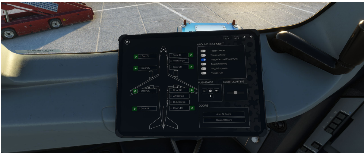
Ground Equipment - Controls doors on the aircraft along with requesting external Ground Services Equipment, Jetway, Pushback, manual steering of the aircraft during pushback, Closing & Arming of the Doors and Cabin Lighting.
