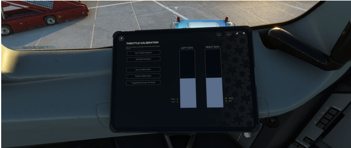
Throttle Calibration – This page allows you to set and calibrate our throttle positions.
