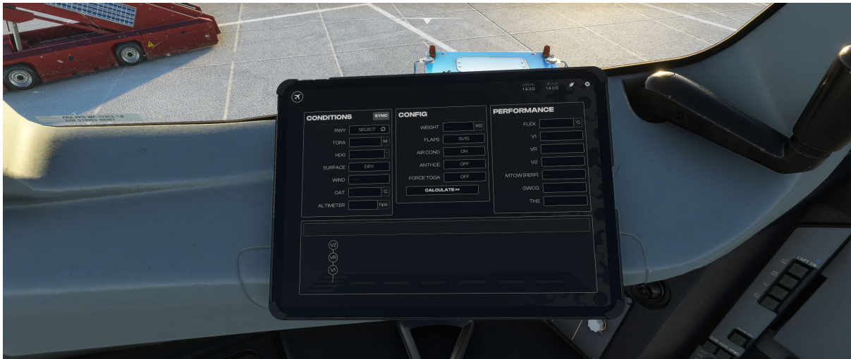
Performance - This page allows you to set the conditions for Takeoff to calculate your performance references.
