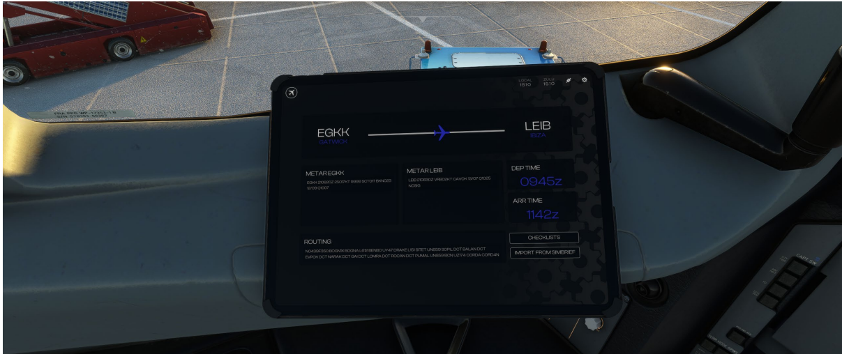
My Flight – Shows your current flight details as set in the FMS and routing details along with METAR for your departure and arrival airports. You can import your flight details directly from SimBrief. You can also access the Checklists from this page.
